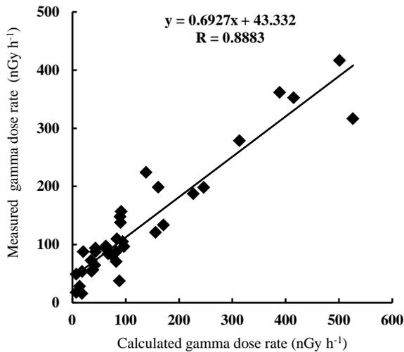
**Fig. 5.** Relationship between directly measured dose rates and dose rates calculated from concentration of  $^{226}\text{Ra}$ ,  $^{232}\text{Th}$  and  $^{40}\text{K}$  in soil samples from Belitung
