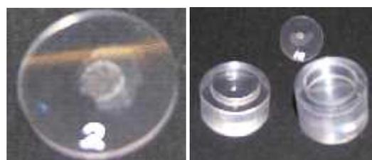
Fig. 5. Plastic Scintillation.
