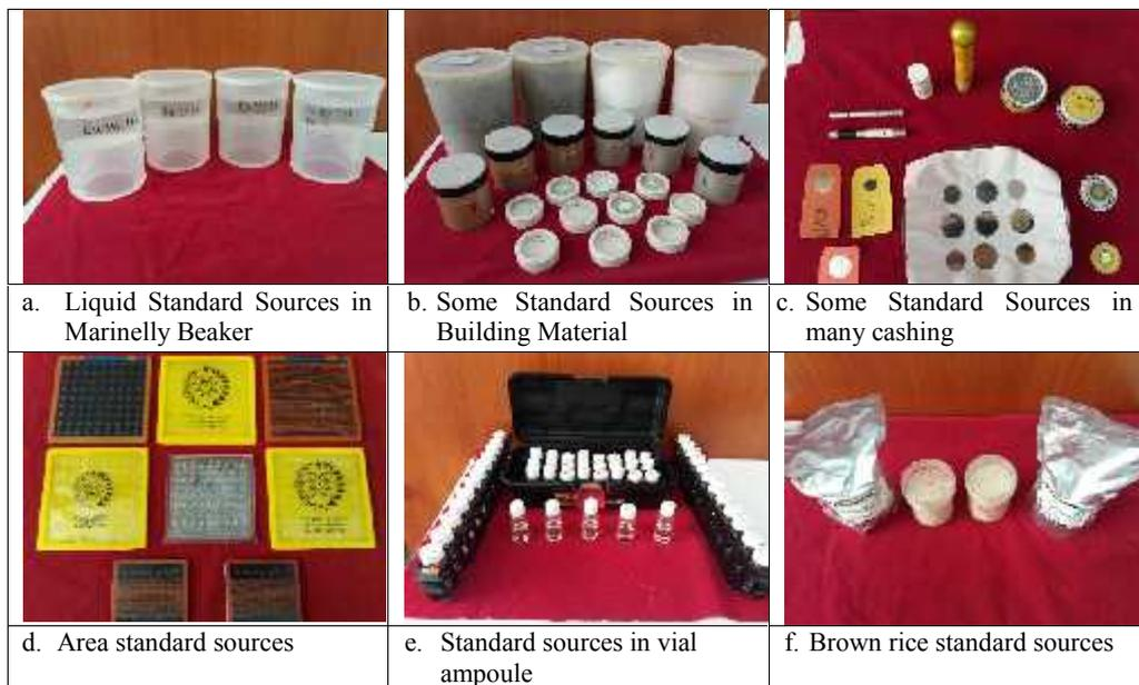
Fig. 6. Many kind and type of standard sources made by PTKMR-BATAN
