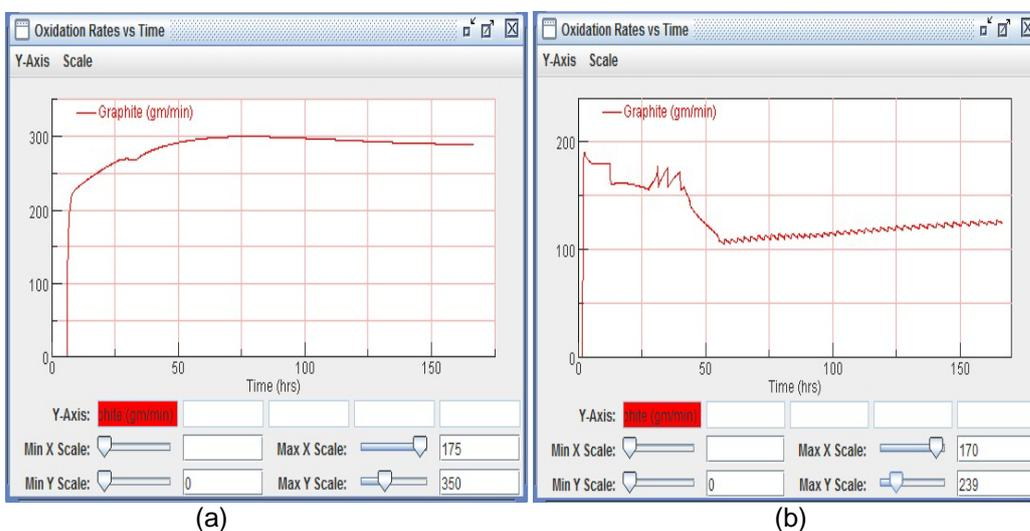
**Figure 4.** The rate of graphite oxidation predictions versus time on condition ATWS.
