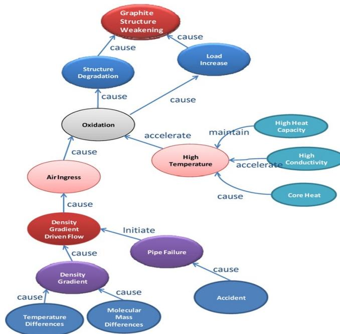
Figure 1. Root causes of air-ingress accident [17,19]
