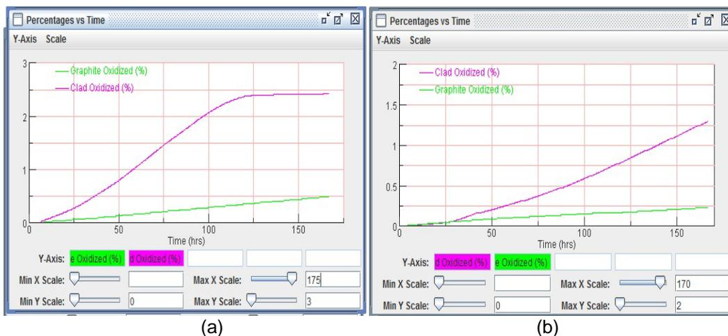
**Figure 5.** Fractional weight loss due to oxidation versus time on condition ATWS
