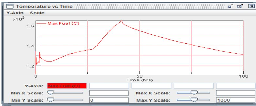
**Figure 3.** Fuel temperature vs time with delayed ATWS conditions for 2500 minutes on D-LOFC condition
