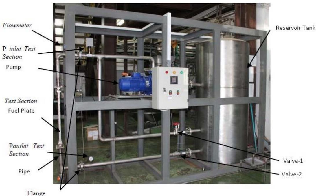
**Figure 2.** The Channel Experiment Facilities (ExNal) [1]
