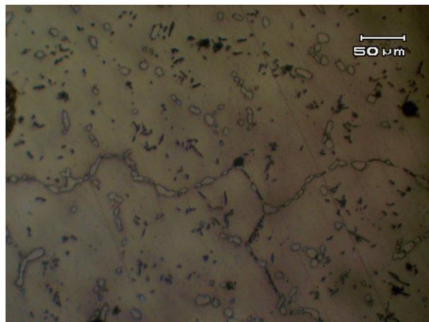
Figure 2: Optical micrgram of new ferritic sampel after homogenization at 1200°C for 20 h.
