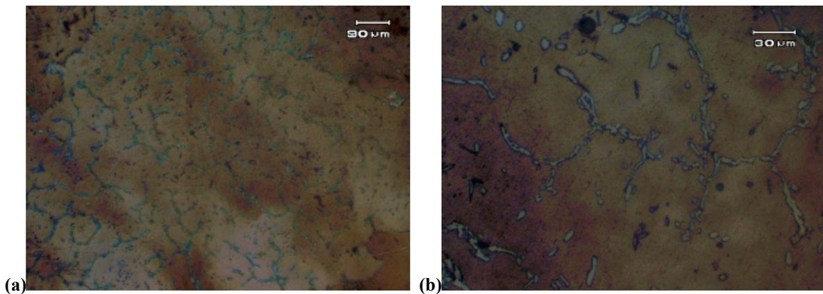
Figure 1: Optical Micrograms of original ferritic ingot. Sample was made by foundry method.
