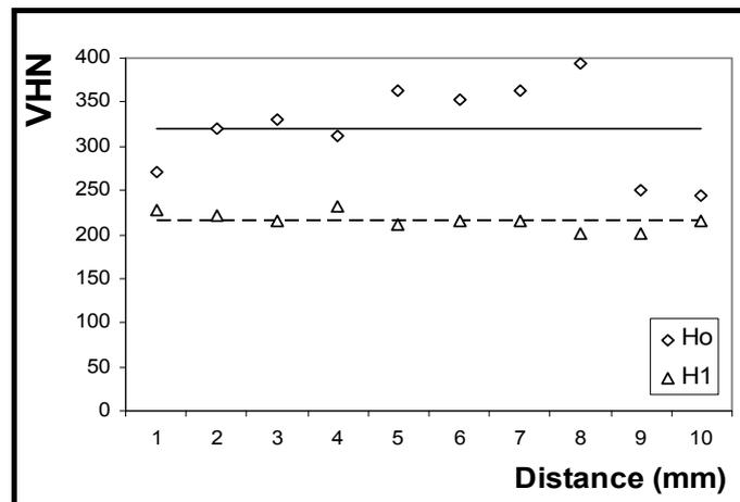
**Figure 4:** Ingot Vickers hardness number; the lines shows the average material hardness value respectively; Ho and H1 shows material hardness before and after homogenization respectively.
