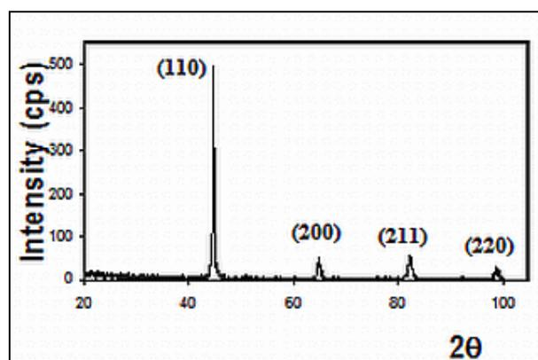
Figure 3: F1 ferritic material X-ray diffraction pattern shows the bcc crystal structure
